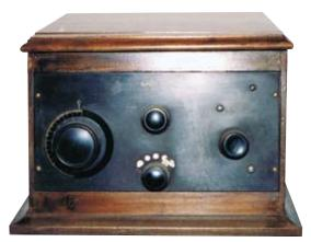
CROSLEY MODEL 51-S – This two tube battery receiver was manufactured in 1925 by the Crosley Radio Corporation in Cincinnati, OH. The "S" in the model number means "Special." The chassis and panel are the same as the standard Crosley Model 51, except for having a variable plate tuning condenser instead of the older "book" type tuner and a larger more deluxe cabinet. (Dave Crocker, Mashpee, MA)
